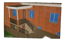
The renovation of the west entry is scheduled to begin after March 1. The renovation will consist of the replacement of the upper and lower steps, a new 10ft x 12ft landing on the upper level, a new roof over the landing, and new entry doors. The completion date is set for June 1, 2020.
